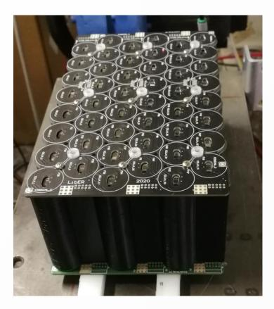
Example of a battery pack made by 48 cylindrical cells, with 96 welding on two sides
