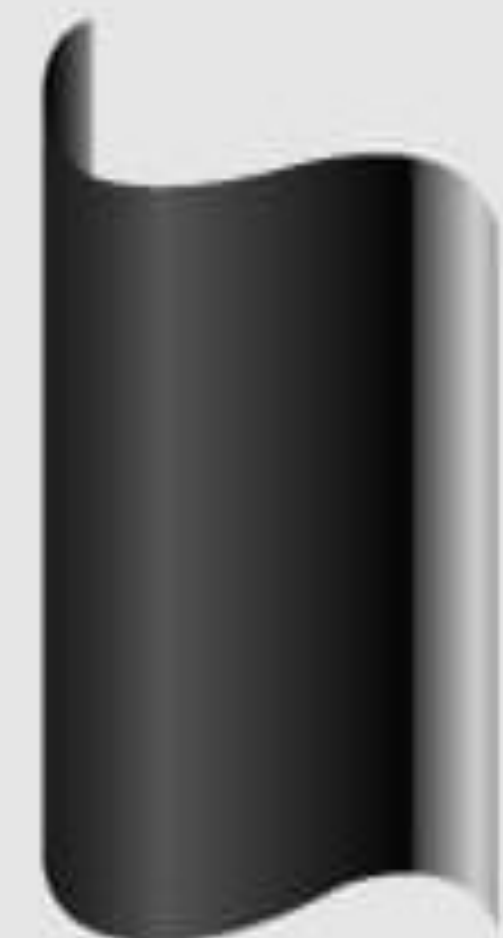
Cathode electrode: Cathode active material applied to the aluminum foil.
