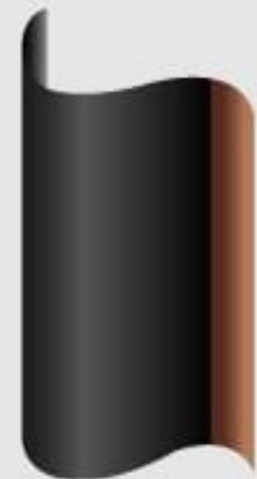
Anode electrode: Anode active material applied to the copper foil.
