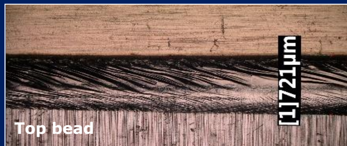
Lamine 2x200 \mu m, 500W >7.8m/min
