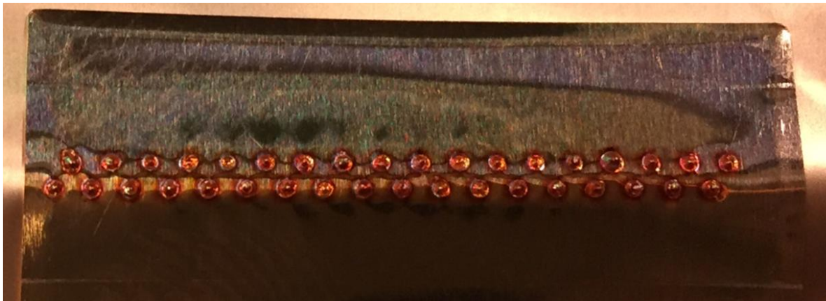
Successfully welded stack of 100 Cu foils (8 \mu\text{m} each) with ARM laser
