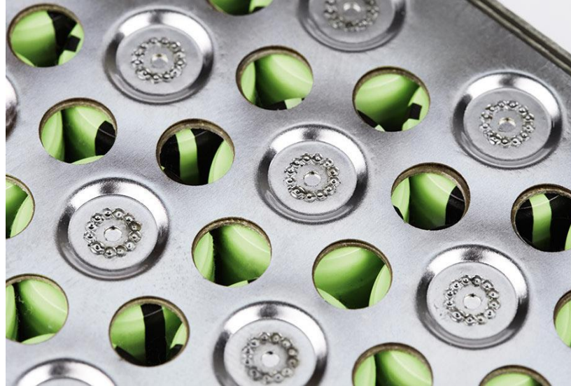
Laser welding on large bus bar
