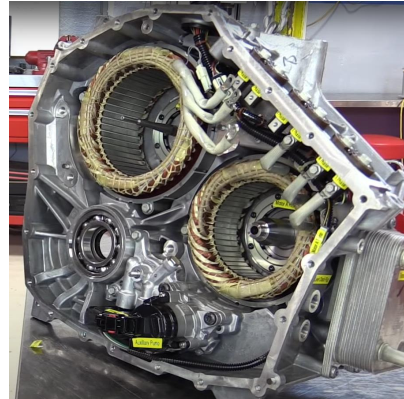
Chrysler Pacifica Si-EVT Hybrid Transaxle
